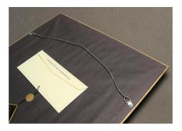
Pictured are medium-weight, single-hole D-rings with #2 coated stainless steel wire. Set the straps about 4 cm down from the top edge of the frame and position the straps so the wire will slant 60 degrees when the picture is set on two wall hooks. Make the wire slack enough to reach halfway between the straps and the top of the frame but so slack that it can be seen when the picture is hung.
