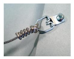
Here you see a medium-weight, single-hole D-ring with a #4 pan-head Phillips screw and #3 coated stainless steel wire. The wire is mounted with a lark's head knot, twisted tightly and compressed where it attaches to the D-ring to prevent the wire from slipping.
