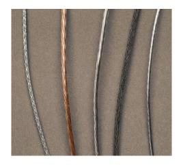
(left to right) #5 twisted stainless steel, #9 coated copper, 36 plastic-coated stainless steel, #6 multistrand braided galvanized steel, #4 plastic-coated twisted stainless steel
